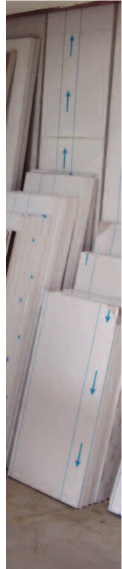
Strippable plastic film typically indicates the rolling direction.
