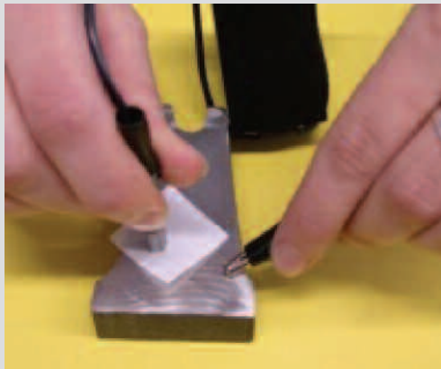
Easy-to-use electro-chemical test methods are available to find out whether a stainless steel grade is molybdenum-containing (left) or not (right).
