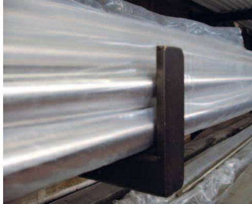
The plastic packaging protects the stainless steel hollow sections against iron pickup from carbon steel racks.
